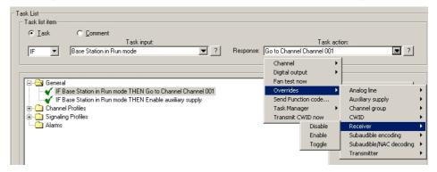
The first two lines are executed as soon as you activate the input. The receiver is disabled and the timer (used to re-enable the receiver) is stopped. If you deactivate the input, this starts the timer (third line). When the timer times out (after 150 ms as long as you don't activate the digital input), Task Manager enables the receiver (fourth line).
