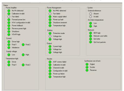
You can configure the base station to disable any alarm that is inappropriate for your system. For example, the External reference alarm is only suitable if the TB9100 expects a to have an External frequency reference. Disabled alarms appear gray on the Current Status form, do not activate the control panel alarm LED, and are not listed in the alarm log.
