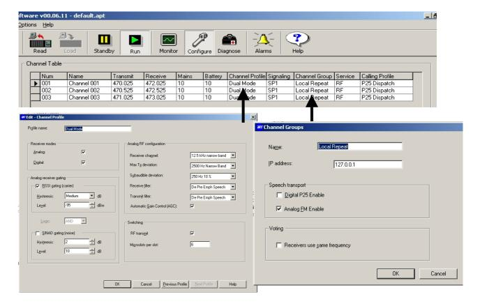
Custom profiles make it possible to maintain sets of completely different configurations and to switch between them. For example, one channel could be set up as a repeater and another as a line-connected base station. All that is needed to convert the TB9100 from a repeater to a line-connected base station (or vice-versa) is to change the operating channel. You can define up to 16 channel profiles and 16 signalling profiles.
